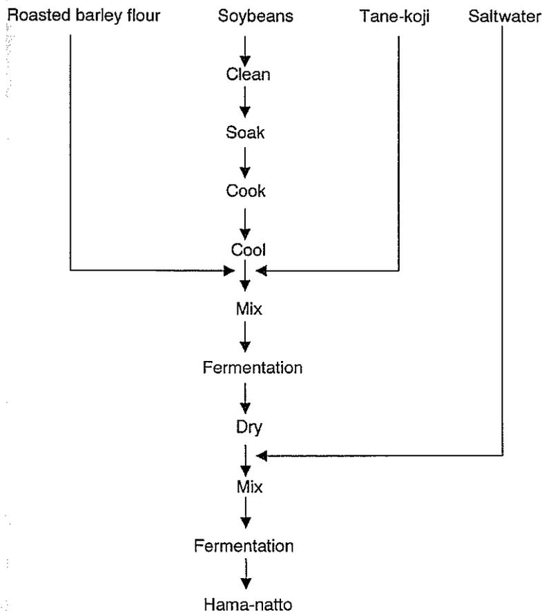
Figure 8 A flow diagram for the production of Hama-natto.
